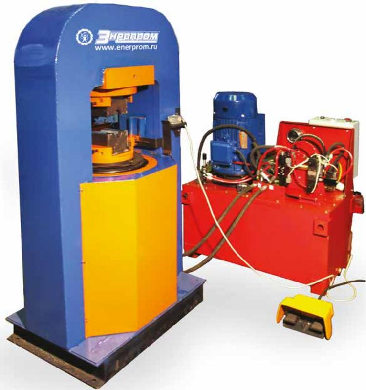
with crimped aluminum alloy plugs and provide the geometry of the pressed plug with guaranteed removal of the flare due to the rigid structure, the required standard force and the exact positioning of the matrices.
